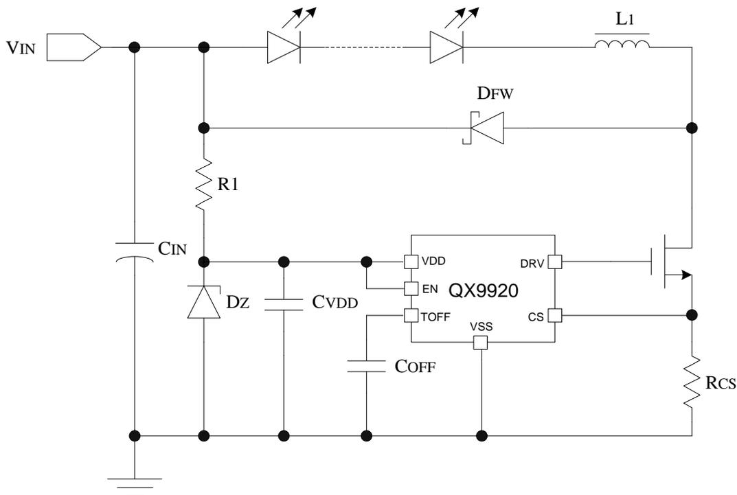
Figure 1: Typical Application Circuit Diagram of QX9920
