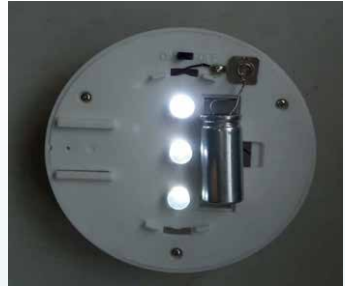
PV panel+ICC supercap+LED light
